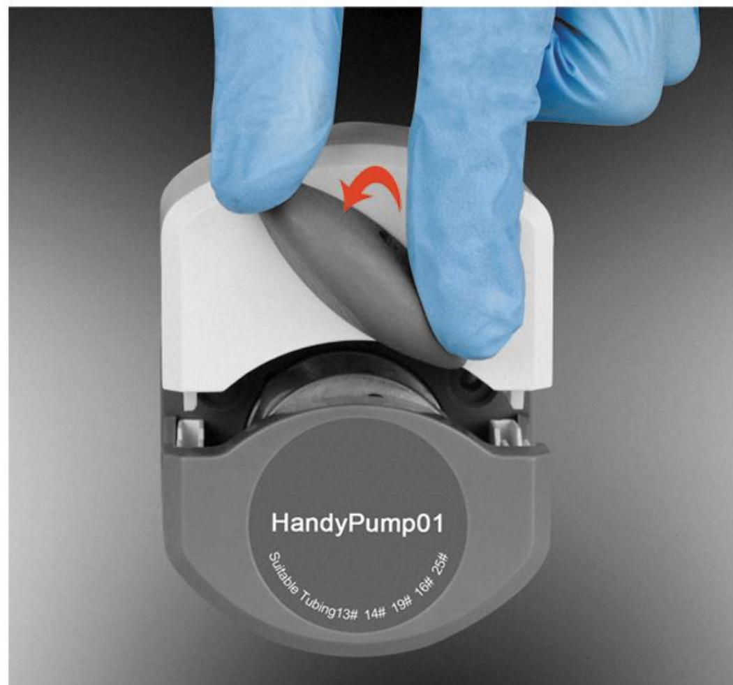
1. Turn the knob anticlockwise 180°, open the upper block.
