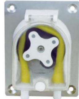
D. Close the transparent cover, and turn the holding pin to unlocking position.
