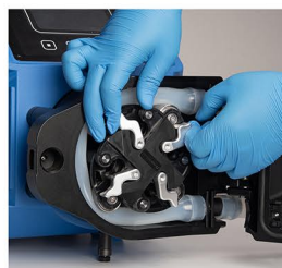
4. Rotate the roller assembly and move the rollers into the working position using the lever.
