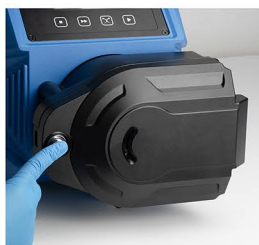
2. Press the locking switch to open the pump head.
