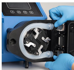
3. Install the built-in tube assembly into the pump head and press the tube connectors into the corresponding grooves.
