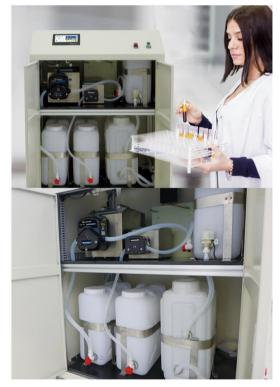
Application 3 Medical industry: automatic liquid mixing system, intelligent proportional mixing of different liquids, the system can intelligently detect the liquid level of the barrel. Through the analysis of the liquid state of each barrel, control the start and stop of the peristaltic pump, open and close OF solenoid valve, so as to realize the automation of the work flow.
