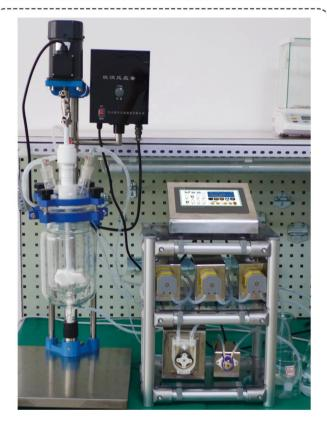
Application 4 Bio-pharmaceutical: Work with reactor or fermentation tank, the OCM system add different liquids with proportion and order into reactor.
